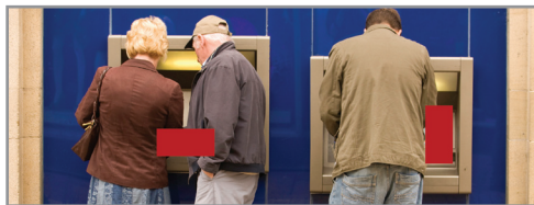
The Privacy Mask Function blocks certain sensitive areas of the camera view (such as ATM keypads) while still allowing a full field of view.
